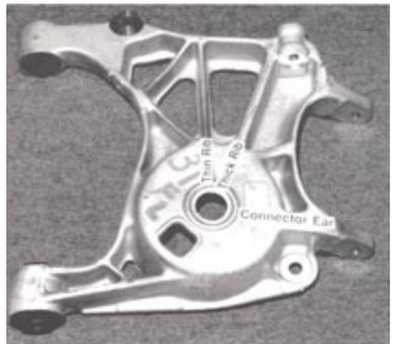
**Figure 1.** A356-T61 Lincoln Mark VIII Cast Lower Suspension Control Arm
