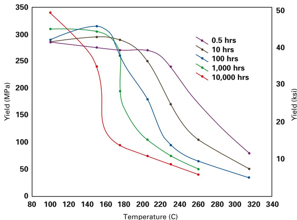
**Figure 5.** A plot of Yield Strength versus temperature for 354-T6 as a function of exposure time at temperature before testing at temperature.
