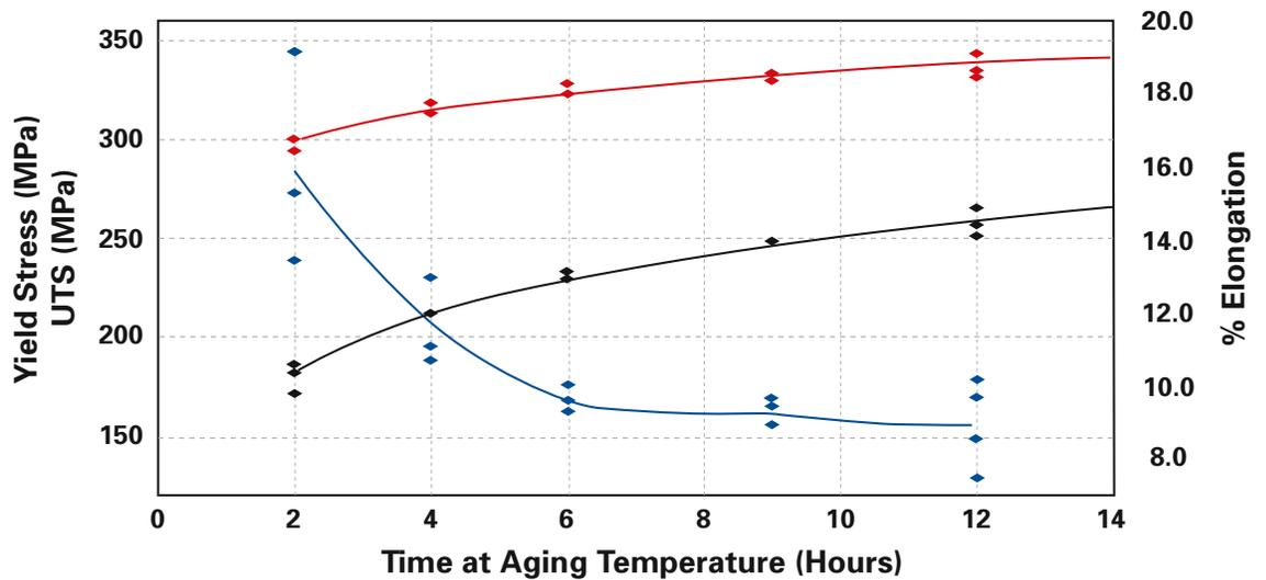
**Figure 3.** Typical Aging curves for A356-T61 separately cast tensile bars. Aging temperature was 155°C. Note that 170°C is sometimes used for faster aging when accurate time controls are in place.
