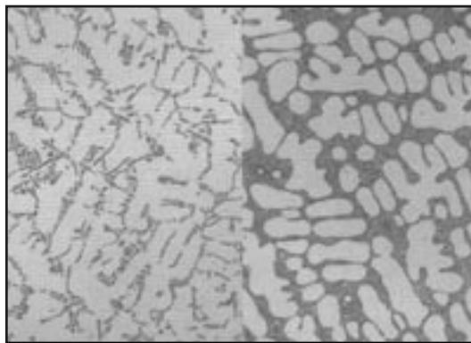
**Figure 7.** Modified (right) versus unmodified (left) microstructures.
